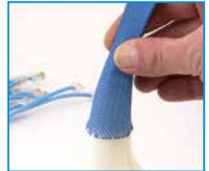
To install the sleeving over your application, just push the flared end over the ends of the wires and "walk" the sleeve down the length of the bundle from behind. Once the sleeving is in place, just run your hand over the applied sleeving to smooth it out.
