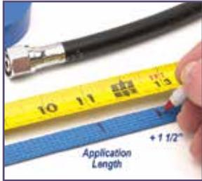
Measure the sleeving and mark the measurement with a pen or marker. Add an additional 1 1/2 - 2 inches and cut the extended length of sleeving.
