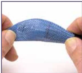
Slip the additional length of sleeving over the end of your application so that the mark is at the spot on the installation where you want the sleeve to end. On this low pressure air hose, it's just below the connector.
