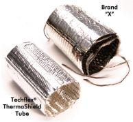
Techflex<sup>®</sup> ThermaShield<sup>®</sup> and a competitor's similar product were placed in the same electrical test oven for one hour at 626°F (330°C). Note the burning and delamination of the fiberglass interior of the Brand "X" product. Even the metallic shroud suffered a degree of burning and brittleness that did not occur on the ThermaShield<sup>®</sup> sample.
