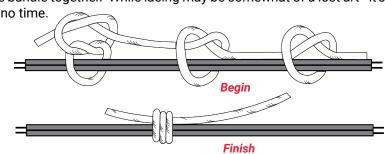
Once the knot is made, you simply make a series of lock stitches along the length of the bundle in equal intervals, again pulling tight as you go.
